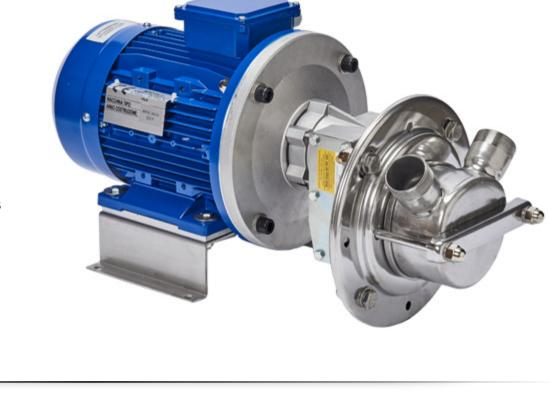
■ Immediate priming at a depth of up to 5 metres, even when running dry Flow reversibility ■ Motors compliant with IEC 72 UNEL-MEC standards, widely available in all national and international markets should they need to be
